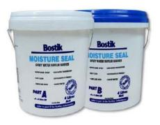
Bostik Moisture Seal (BOSMS) - is a 2 part water based epoxy coating designed as a moisture and vapour barrier membrane to prevent water seepage and permeation through concrete floors. The product shows excellent adhesion and acts as a surface preparation for subsequent adhesives when laying floor coverings of all kinds.
