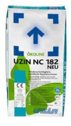
Uzin NC 182 (UZNC18220) - Trowel applied strength, rapid cure floor levelling compound. Water mixed (5-6L water). Feather edge—100mm low slump. Very fine surface finish. Interior use only. Recommended that all substrates should be primed. Can be covered after 1 hour. 30 MPA
