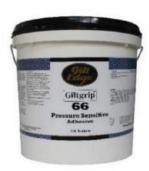
**Giltgrip 66 (GG66)** Giltgrip 66 Pressure Sensitive adhesive is low in VOC and has been developed for the installation of vinyl composition tiles. It is also suitable for the installation of carpet tiles and slab underlay's used in the double bond carpet installation. It has good plasticiser resistance.
