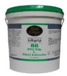
**Giltgrip 88 (GG88)** Giltgrip 88 PVC Tile & Vinyl Adhesive is a high performance, low VOC, acrylic based adhesive specifically designed for the installation of PVC planks and tiles. It is also ideal for the installation of commercial and domestic sheet vinyl. This low VOC formulation exhibits excellent plasticiser resistance and is formulated to provide quick initial grab. It is **not** recommended for the installation of linoleum.
