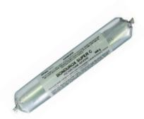
**Giltgrip Super C (UGGSUPC600)** - A single pack high strength low foaming moisture curing polyurethane based adhesive. Bonding most types of resilient and rubber flooring/underlay/acoustic products to concrete and timber substrates. Due to the highly variable nature of rubber and resilient products in the market, contractors should test lay a typical sample and do a destructive pull test to confirm adequate adhesion to a given substrate.
