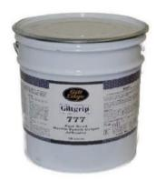
**Giltgrip 777 (GG777)** Giltgrip 777 is a solvent based trowel applied adhesive for bonding synthetic backed carpet on to concrete or timber. Giltgrip 777 has an exceptionally strong initial grab and gap filling to ensure the best possible bond to most interior surfaces. It exhibits good water resistant bonds and water damage even after 5 hours will not affect the bond even if the adhesive becomes flooded.
