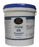
**Giltgrip 22 (GG22)** is a water-based Latex adhesive with low VOC and has been specifically formulated to provide extra open time for positioning of long runs of commercial carpet before it develops its "leggy" grab and holding power for jute & action backed tufted carpets, woven wilton & axminster carpets and most needle-punched carpets.
