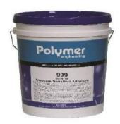
**Polymer 999 (R999)** Polymer 999 Pressure Sensitive is a pure acrylic solvent free, non staining co-polymer adhesive designed to provide a permanent tacky pressure sensitive film. For bonding carpet and vinyl floor tiles where a re-peelable job is required. Also used for the installation of slab rubber carpet underlay used in the double stick installation system.
