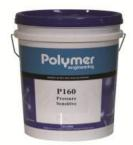
**Polymer 160 (R160)** A latex based pressure sensitive adhesive offering economy prolonged open time and excellant adhesive properties. For multiple application including but not limited to: double-stick underlay installation, direct stick carpets seagrass and coir installations and commercial vinyl tiles. It is particularly suited to lower temperature installation (between 3-10°) where acrylic type products are very slow to tack up.
