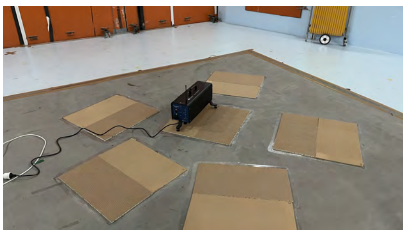
Figure 2.8: 5.5 mm sample under test showing tapping machine
