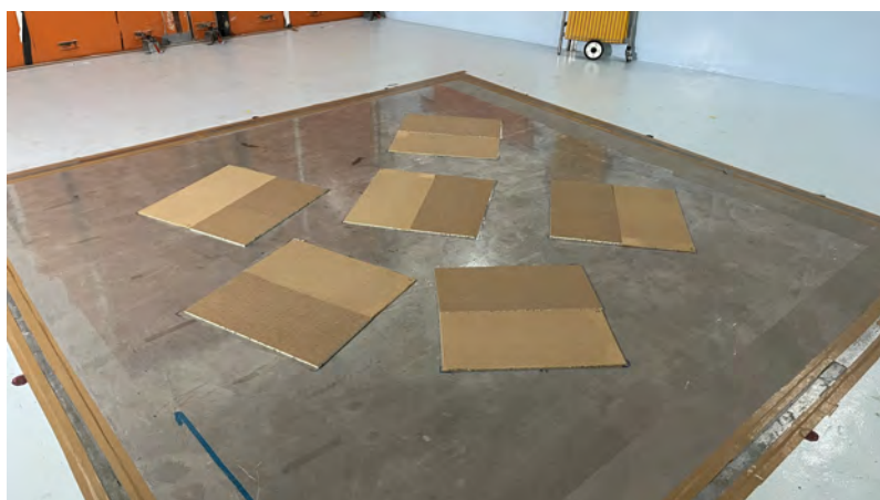
Figure 2.7: Underlay samples applied and ready for testing
