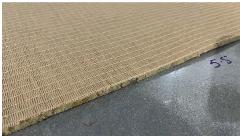
Figure 2.3: Giltgrip Double Bond 5.5mm foam chip underlay surface detail
