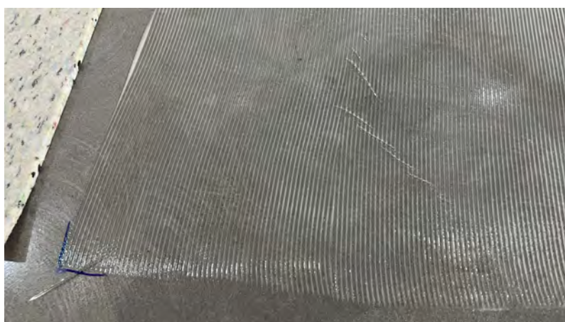
Figure 2.6: Giltgrip 66 adhesive ready to apply samples
