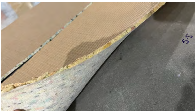
Figure 2.4: Giltgrip Double Bond 5.5mm foam chip underlay section/base detail
