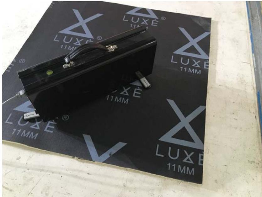
Figure 1: Tapping machine on sample in position 1
