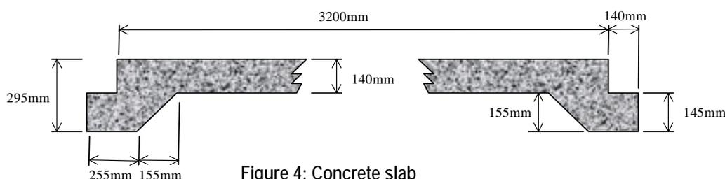
Figure 4: Concrete slab
