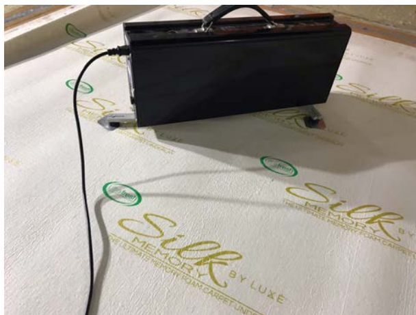
Figure 2.2: Underlay detail with tapping machine positioned in chamber
