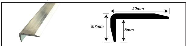
Timber Angle Ends are used as an edge capping for your new timber floor and covers the expansion gap between the floors and walls, carpet, sliding doors and entrance mats.
