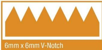
Trowel size is suggested to maximize coverage of adhesive. Periodically lift a board to insure the following conditions are being met: 100% coverage of concrete substrate and 100% transfer to the back of the flooring product. Uneven subflooring may require the use of either a levelling/patching material, or a larger V-notched trowel for proper coverage of adhesive.
