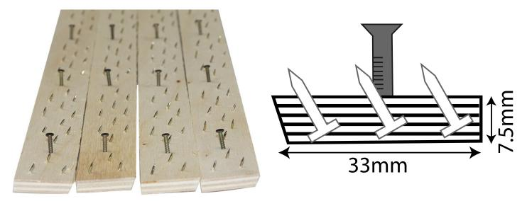
Offers a full 3 rows of pins set in a 32mm wide plywood strip. Has added advantage of being suitable for wood or concrete installation. An economical alternative to double stripping and full width commercial carpet strip. Provides extra insurance on difficult residential installations.
