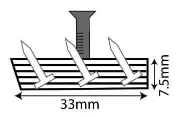
Offers a full 3 rows of pins set in a 33 mm wide plywood strip. An economical alternative to double stripping and full width commercial carpet strip. Provides extra insurance on difficult residential installations
