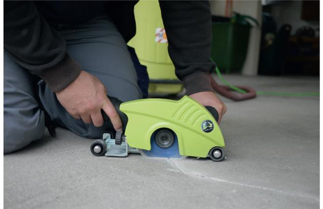
Simply expand screed cracks, joints and set cross-sections with little dust, using the Scred Joint Cutter from Wolff Tools.
