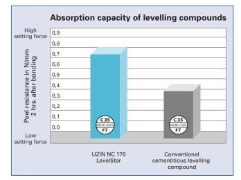
The absorbency of the new premium levelling compound is approx. twice as high as previous levelling compounds. The open time of the adhesive during the laying is considerably reduced in comparison with usual compounds. The installer of the covering works far faster and the overall appearance of the finished floor covering surface is very smooth and flat.
