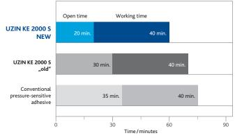
PVC sheet installation on UZIN NC 170 LevelStar, notch size A 2, at 20  $^{\rm o}{\rm C}$  and 65 % relative humidity.
