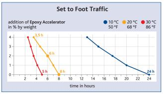
An addition of 2 % allows two coats to be applied within one day.
