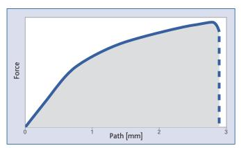
The curve for the UZIN Turbolight®-System also rises steeply, indicating the system's low level of deformation. The displacement that occurs at higher loads reveals a very well-tempered response with high levels of load compensation and reserves, as a result of the energy absorbed (grey area).
