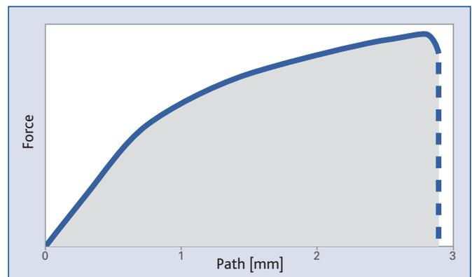
The curve for the UZIN Turbolight®-System also rises steeply, indicating the system's low level of deformation. The displacement that occurs at higher loads reveals a very well-tempered response with high levels of load compensation and reserves, as a result of the energy absorbed (grey area).
