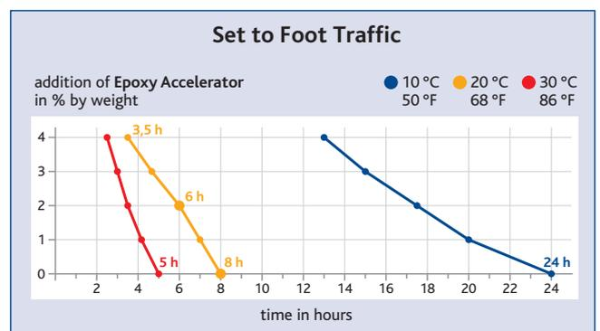
An addition of 2% allows two coats to be applied within one day.
