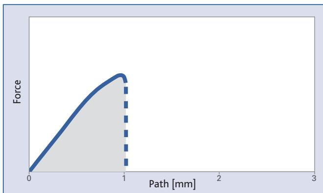
When subjected to a pressure test (based on DIN 18 555), the substructure, consisting of UZIN NC 194 Turbo and UZIN NC 170, shows a steeply rising curve. The curve terminates abruptly, i.e. the combination fails because of a brittle fracture. The area under the curve (grey), defining the energy absorption capabilities of the substructure, is relatively low.
