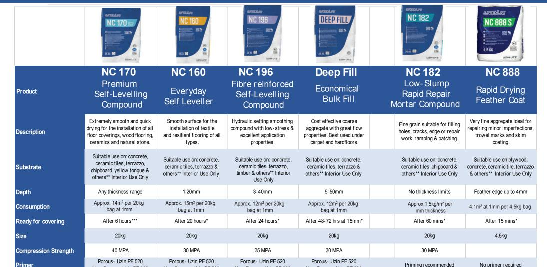
\*At 20 °C and 65 % relative humidity; \*\*Refer to product data sheet; \*\*\*At 20 °C and 65 % relative humidity at max. 5 mm thickness NOTE: The substrate must be sound, load-bearing, dry, free from cracks, clean and free from materials (dirt, oil, grease), that would impair adhesion. Cement and calcium sulphate screeds must be abraded and vacuumed and in some circumstances primed. Test the substrate in accordance with applicable standards and bulletins and report any deficiencies.
